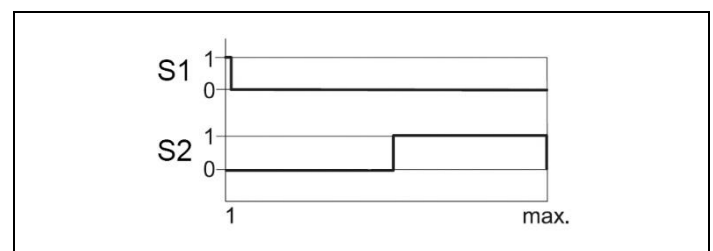
Figure 11: Signal course - clamping
