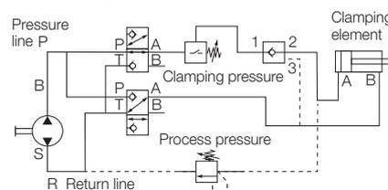
For safety reasons and in the sense of the machine tool guide lines ML2006/42/ EC the hydraulic pressure must be maintained.
