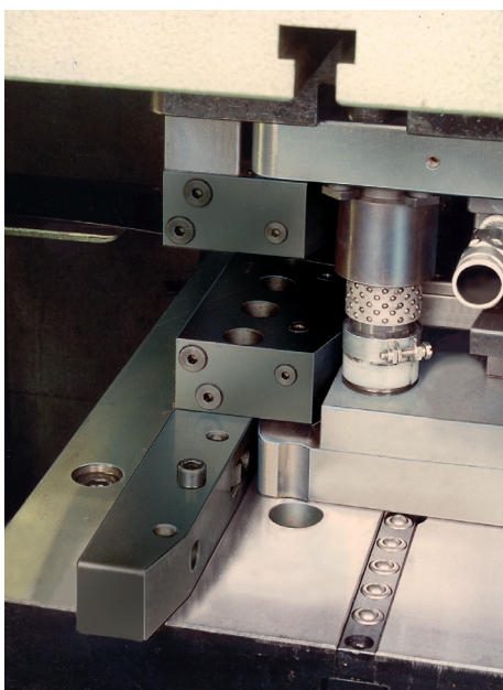
Retrofit to an existing double-column press. Die insertion facilitated by chamfered spacer bars and ball bars.
