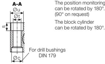
**Installation of drill bushings to absorb side loads**
