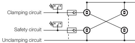
For safety reasons and in the sense of the machine tool guide lines ML2006/42/ EC the hydraulic pressure must be maintained. When upper moulds/dies are clamped by wedge clamps, they must be secured mechanically when maintenance work is carried out.
