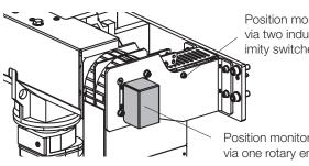
Position monitoring 1 via two inductive proximity switches
