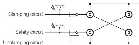
For safety reasons and in the sense of the machine tool guide lines ML2006/42/ EC the hydraulic pressure must be maintained.
