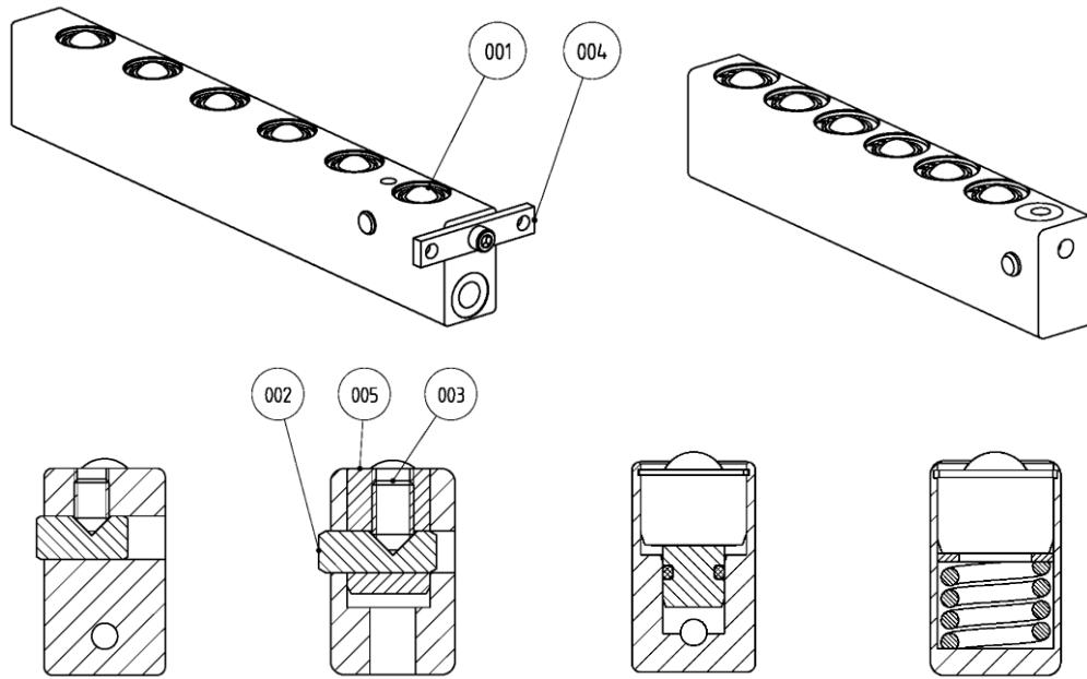
**Hydraulic ball bar: fastening plate (R) / Wedge lock (K)**
