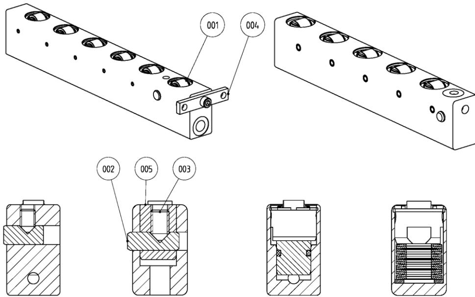
**Hydraulic roller bar: Fastening plate (R) / Wedge lock (K)**
