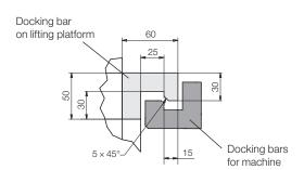
**Docking bar light** simplified docking bar for fixing at the machine/press L = 500 mm
