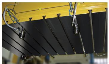
Rapid clamping system with pneumatic cylinder
