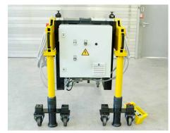
Option: The control is directly mounted to the console, console and control can be completely removed.
